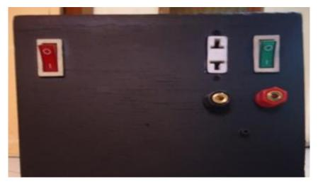
Plug in the main plug of the project. Switch on the green switch for soldering process and when it needs troubleshooting and vacuum is needed, switch on the red switch to open the vacuum motor. For sipping the scrap soldering lead, press the push button switch that is located on the soldering iron handle. Unpressing the push button switch will stop to sip.
